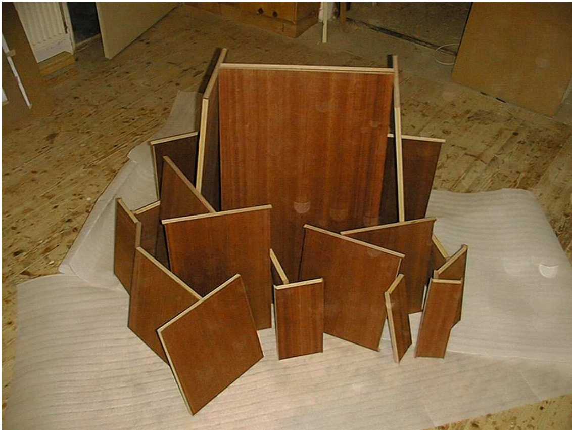
All used wooden parts after veneering and lacquering
