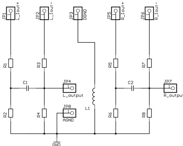
You can see that it is a mix-up of some portion of everything mentioned above: Both output currents are converted to voltage by two small value resistors in series while the straying HF dirt is kept outside the Audio input by a choke (ferrite bead) and only one signal current output – the inverted one - is used.
